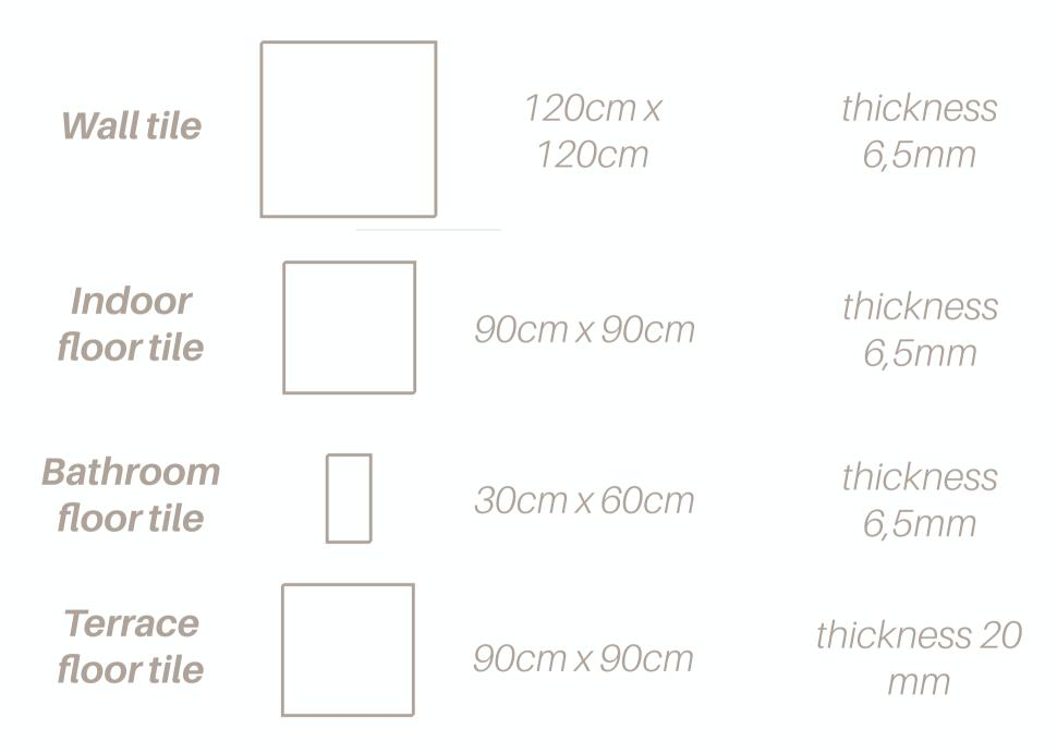
In the interior, all tiles are of the same thickness (6,5-9mm), while in the exterior, such as the outdoor terrace, the large-format tiles of 2cm are stabilized on paving support pedestals. Specially manufactured tiles surround the pool with bull-nose coping.
